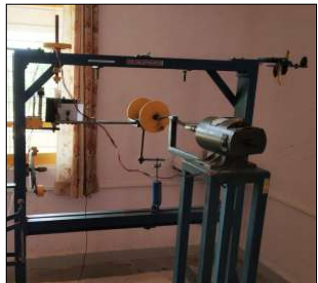
Fig.5 Experimental Setup of Cantilever beam with spring-mass-damper
