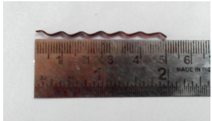
Fig -1: Crimped Shaped steel fibers.
