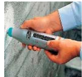
Photo -3: Non-Destructive Test [NDT] on Column and Slab in Building.
