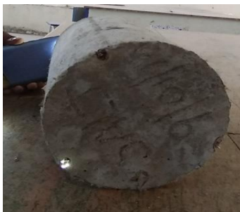
Fig -2: Light Transmittancy Through Cylinder Specimen
