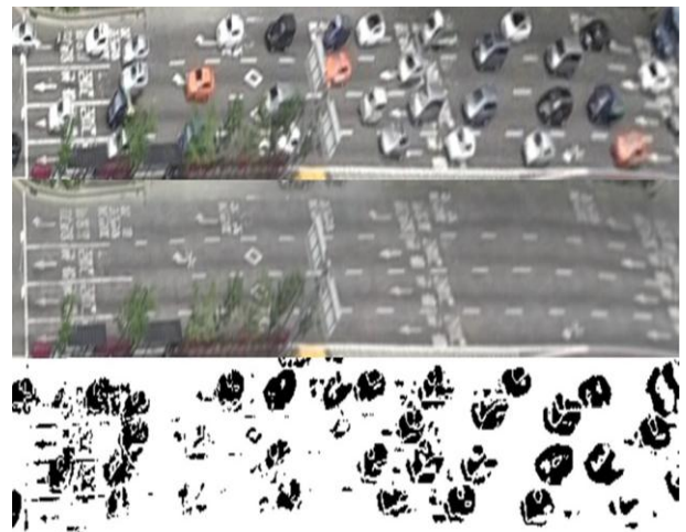
Fig -2: Original and Background subtracted image
