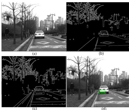
Fig -1: Edge Detection of a vehicle in the road
