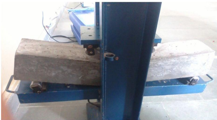
Fig -2: Test Set Up For Flexure Strength Test
