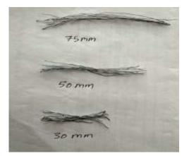
Figure 1: Steel fiber of crimped shape with different length
