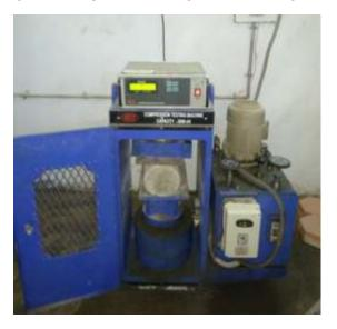
Figure 3: Compression testing machine testing of cylinder
