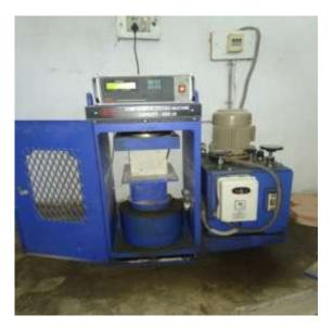
Figure 2: Compression testing machine testing cube
