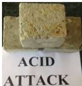
Fig.-1: Specimens subjected to chemical attack
