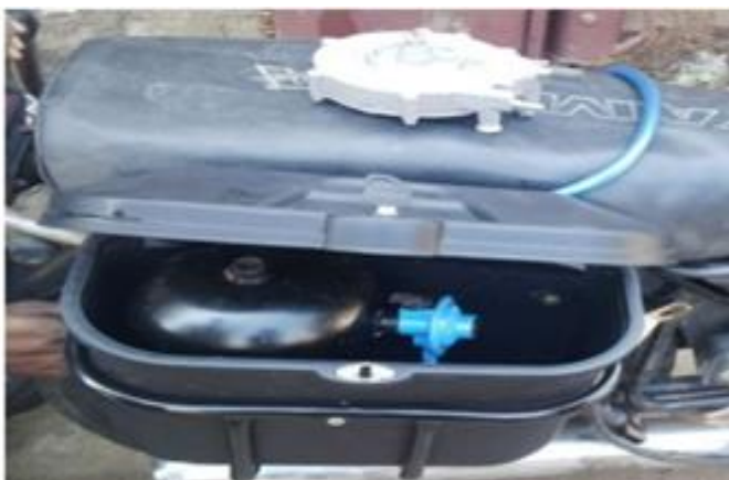
Fig. No. 1 Gas cylinder arrangement
