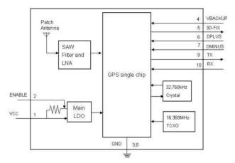
Fig:1.5.2:Block Diagram Representation OF GPS
