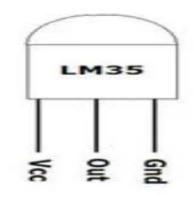
Fig:1.2: LM35(Temperature Sensor)
