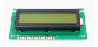
Fig:1.5.3:Liquid crystal Display(LCD)
