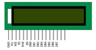
LCD (Liquid Crystal Display) screen is a display module of an electronic device and has a wide range of applications. A 16 x 2 LCD display can be used to display 16 characters per line and there are 2 such lines. It is used to enter the mileage and to display the actual distance to be traveled by the vehicle driver.
