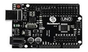
This board contains all the required support needed for microcontroller. They are simply connected to a computer with a USB cable or with an AC -to-DC adapter
