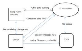
FIG -1: Core Architecture
