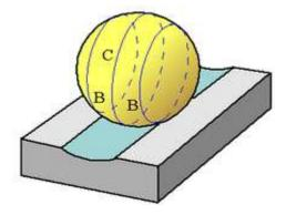
Fig. 3.2: Mechanism of ballizing [8].
