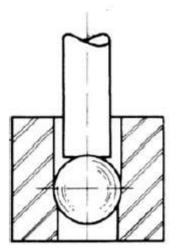
Fig. 3.1: Schematic arrangement of the ballizing process [5].
