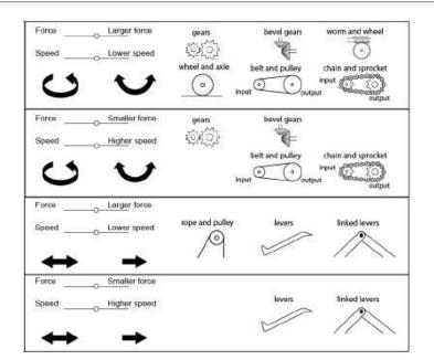
Fig 11:-To Change Output Force and Speed
