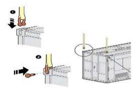
Fig 12:- An example of corner lifting points in containers
