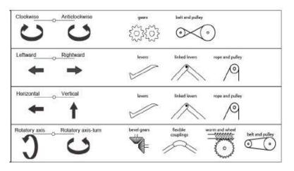
Fig 9:-To Change Direction of Movement
