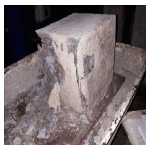
Fig. 9 Non-NFRC cubes spalled after testing
