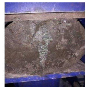
Fig. 10 Bridging Action shown by cylinder
