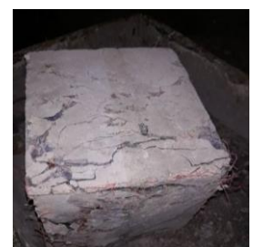
Fig. 12 Post Failure Cracks on Reloading
