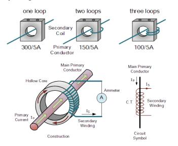
Fig [4] current transformer
