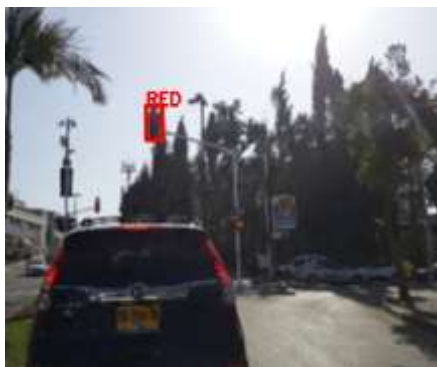
Figure6: Traffic light detection
