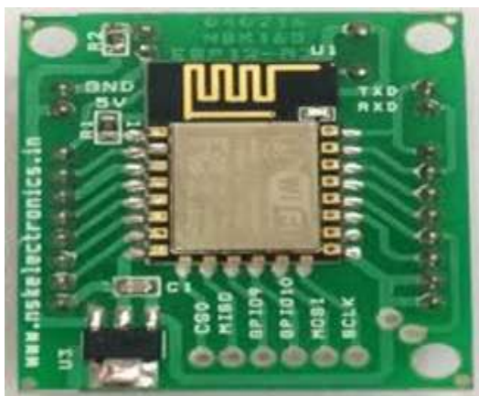
Fig-6: Wireless Transmitter ESP8266
