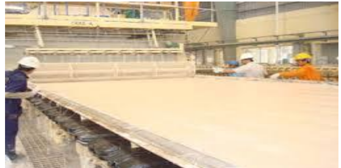
Fig.3: Spreading gypsum plaster for 1 st Layer
