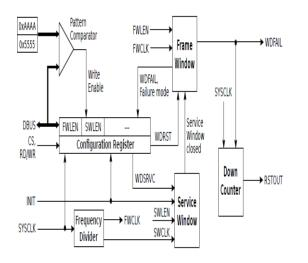
Fig. 6. Functional block diagram of the proposed watchdog timer
