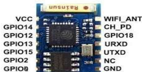
Fig 6: ESP 8266 Pin diagram
