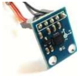
Fig 4: Adxl335 MEMS Sensor
