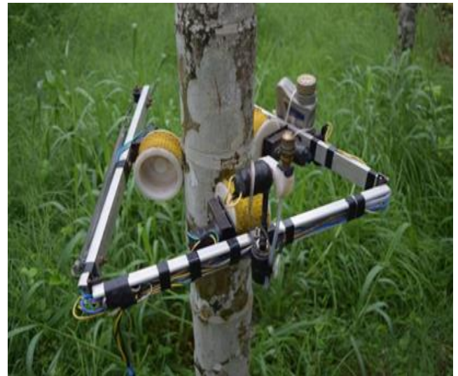
Fig:1 Arecanut tree climbing machine.
