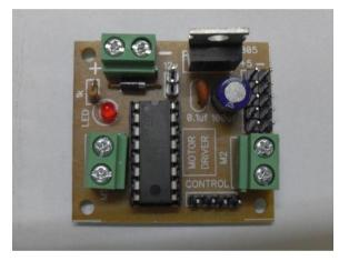
The motor driver is a driver module for DC motors that allows us to control the speed and direction of two motors at the same time. This Motor Driver is designed and developed by considering L293D IC.
