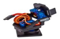
The pan and tilt servo rotates 180° from side to side and can tilt up and downward around 150°. This motor is a plain everyday analog servos we can use microcontroller or driver. The motor helps in fixing the camera when rotating and tilting it up and down.
