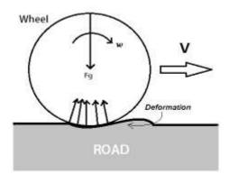
**Fig-3.1.2:** Figure depicting the deformation on the road asphalt due to the wheel's impact.
