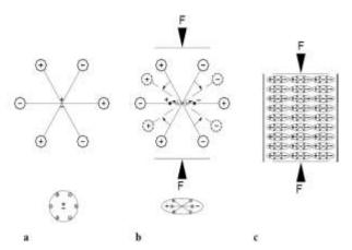
Simple molecular model for explaining the piezoelectric effect: a unperturbed molecule; b molecule subjected to an external force, and c polarizing effect on the material surfaces
