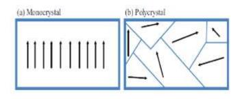
Fig-2.2.2: Structure of Piezo crystals.
