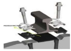
Fig-3.2.1 Implementation of Piezoelectric pads in Railway Tracks.
