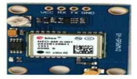
The GPS receiver gets a signal from a GPS satellite. The satellites transmit the exact time the signals are sent. So given the travel time of the **GPS** signals from three satellites and their exact position in the sky, the **GPS receiver** can determine your position in three dimensions - east, north and altitude.
