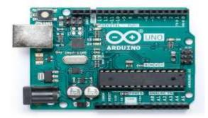
Arduino is an open-source electronics platform based on easy-to-use hardware and software. Arduino boards are able to read inputs - light on a sensor, a finger on a button, or a Twitter message - and **turn** it into an output - activating a motor, turning on an LED, publishing something online.
