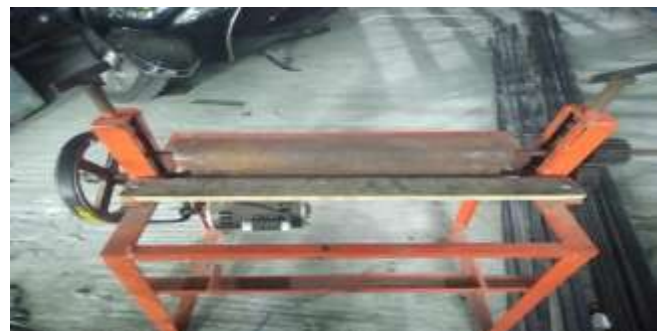
Fig -1: Fibre making machine from banana stem
