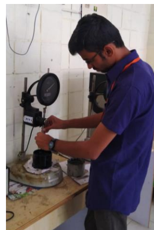
Figure 3 - Penetration Test of Bitumen
