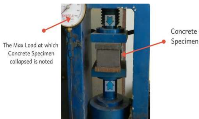
FIG 2: Compressive Testing Machine
