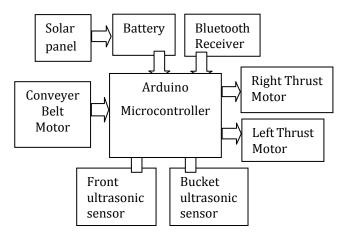
The sun rays incident on solar panel and it convert light energy to electrical energy. This generated energy is stored into the battery, the supply is taken from battery to all electronics and electrical devices. The arduino is the microcontroller it is programmed that it will give command to change the motion of the boat, rotation of conveyor belt etc.
