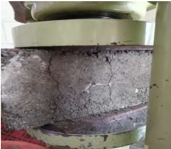
Fig 7. Failure on solid block
