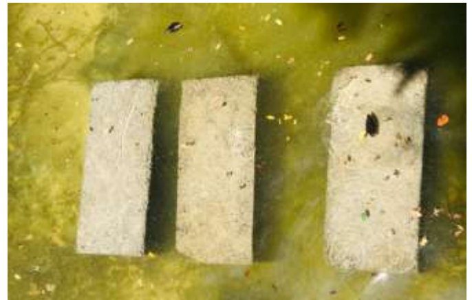
Fig 5. Solid blocks immersed in water for absorption test
