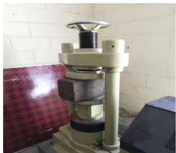
Fig 6. Compressive loading on solid block
