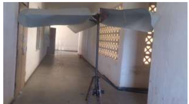
Fig -1: Prototype of vertical axis wind turbine by using spinning top principle
