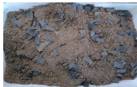
Fig 2.2: Slices of Tyre Mixed With Lateritic Soil
