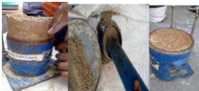
Fig-3: Compaction Test
