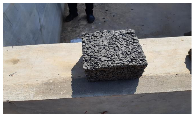
Fig 3-: Curing of Pervious Concrete
