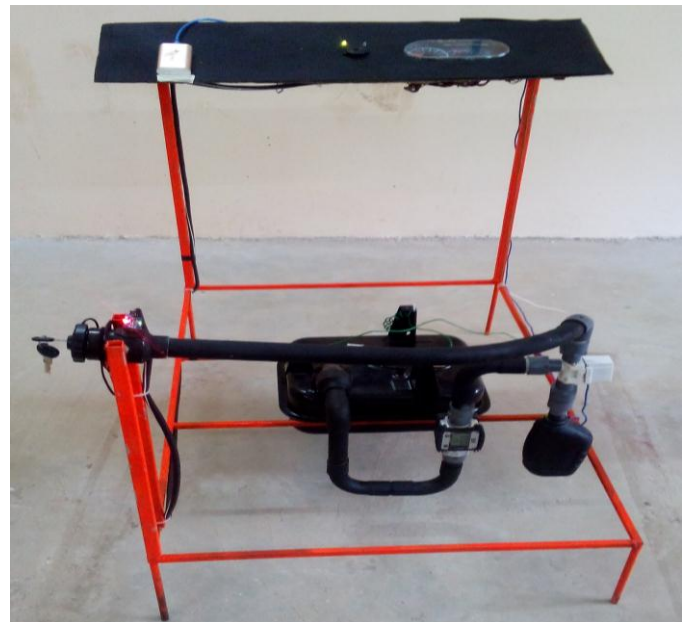
Fig. 12: fabricated model of automated re-fuelling system for automobiles with real – time GPS alerts
