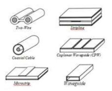
**Coxial cable** --- The coxial cable consist of a central, insulated wire (inner conductor) mounted inside a tubular outer conductor as shown in fig. In some applications the internal conductor is also tubular. The inner conductor is insulated from the outer conductor by insulating material.
