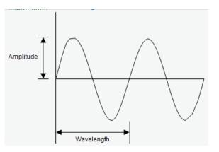
The wavelength of the radio signal is a establishing factor in the size and design of the antenna. Wave length is an actual distance that is usually measured in meters. Ham radio operators often do not refer to frequency band of the radio but use the wavelength to classify the radio. A VHF radio would be mentioned to as a 2 meter rig and a UHF radio would be a 70 centimeter (cm) radio
