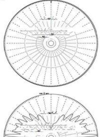
Gia; 6.59 dBi = 0 dB...(Vertical polarization) F/B: -0.16 dB; Rear: Azim, 120 deg, Elev. 60 deg Freq: 145.000 MHz Z: 46.174 + j0.065 Ohm SWR: 1.1 (50.0 Ohm), Elex: 3.4 deg (Real GND; 7.00 m height)
