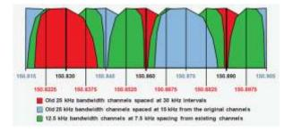
**Further Narrowbanding** --- The FCC has proposed further narrowing the bandwidth of channels below 512 MHz to 6.25 kHz bandwidth but has not issued rules related to a forced migration to this narrower bandwidth at the time of this publication. One of the reasons for this isthelackofFDMAsubscriber equipment
