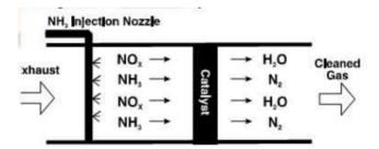
Figure 4: Selective Catalytic Reduction
