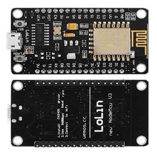
Fig No-2: NodeMCU Front and Back Side
