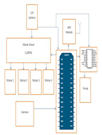
**Dia No-2:** Circuit diagram of Fire Fighting Robot.
