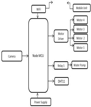
Dia No-1: Block diagram of Fire Fighting Robot.
