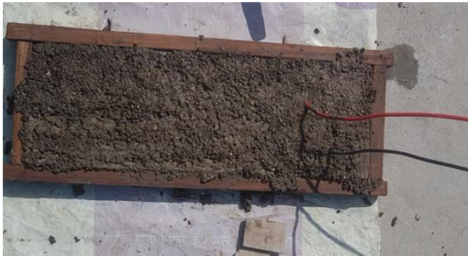
Fig-1: Connection for corrosion monitoring in Ferro-cement panels
