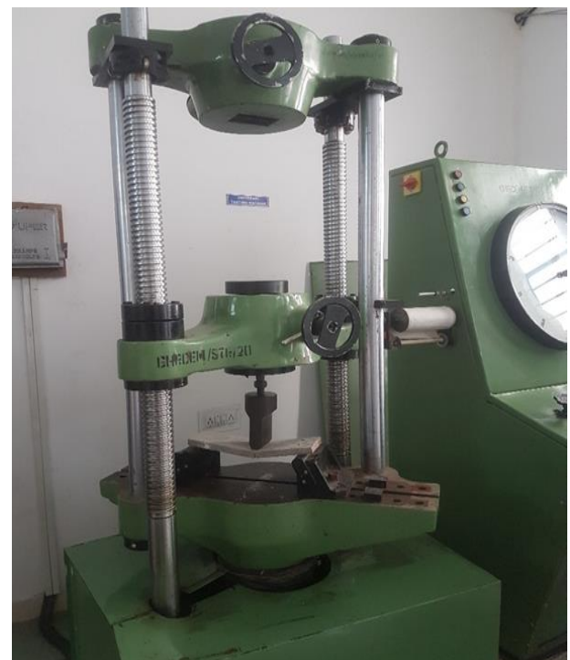
Fig-4: Specimen subject to 3 point loading.
