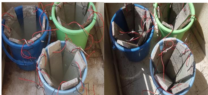
Fig-2: Wetting and drying of specimen in different percentage of NaCL Solution
