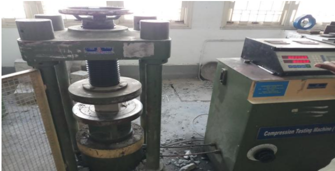
Fig -5: Testing of Cube
