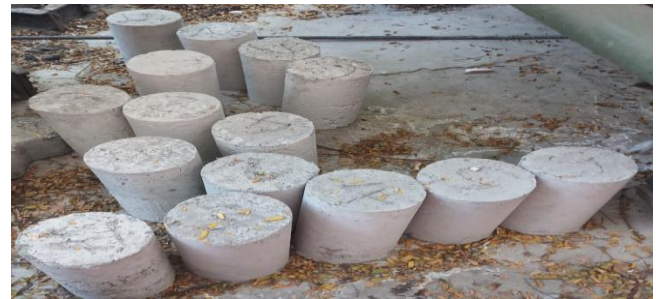
Fig -3: Casting of Cylinder
