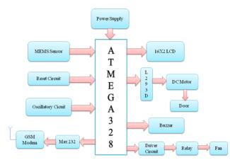
Fig -1: Block diagram representation of Project
