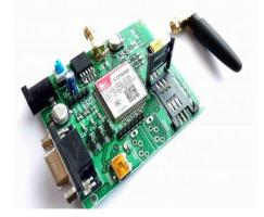
Fig -2: GSM Module
