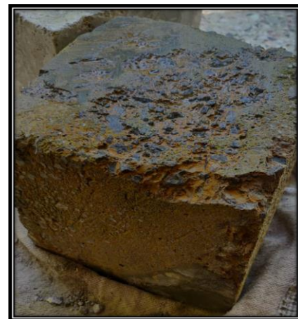
Fig -4: Cube immersed in 5% Nitric acid for 60 days.
