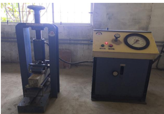
Fig -3: Flexural test on beam
