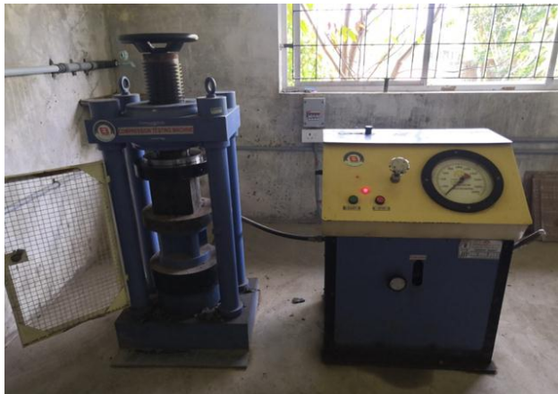
Fig -2: Compressive test on cube
