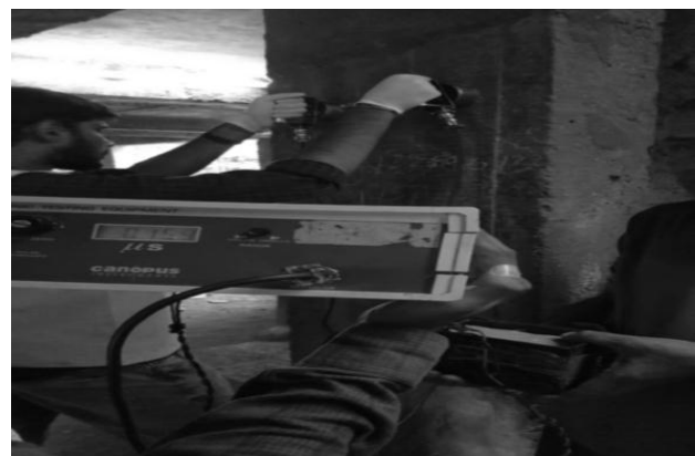
Fig -2: Ultrasonic Pulse Velocity Test
