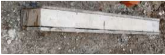
Fig.3.9 Typical Photograph of Beam strengthened with three face confinement
