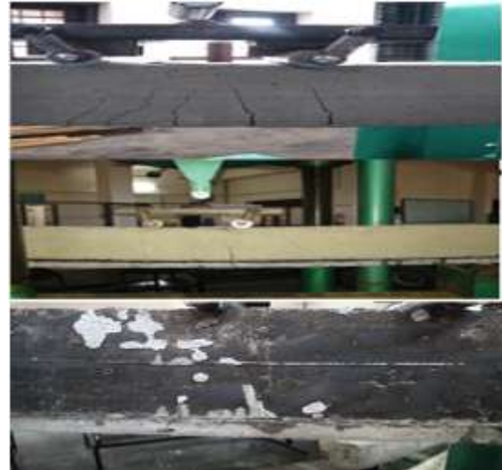
Fig.5.4 Failure Patterns of Beams
