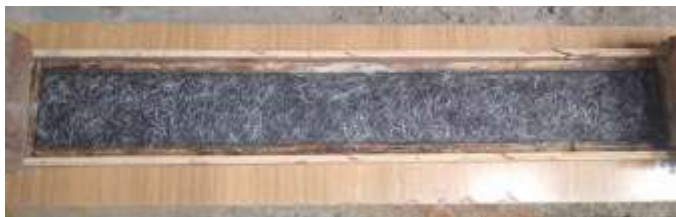
Fig.4.1 Placement of Steel Fibres in a Mould
