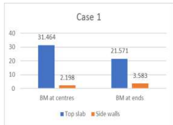
Fig 11. Graph Showing BM at centres and ends of top slabs and side walls for case 1
