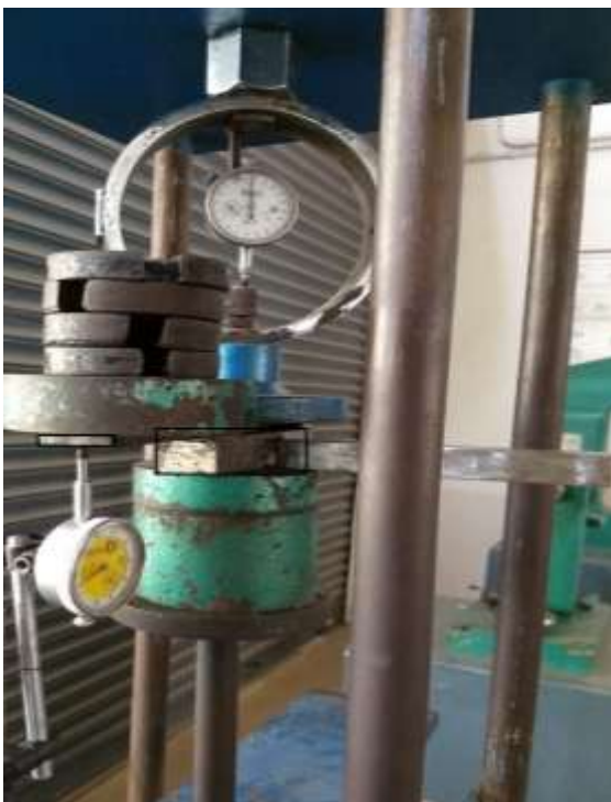
Fig-3.1: Proven Ring Experiment to find the load
