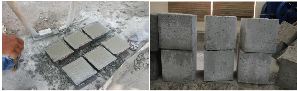
Figure shows casting of concrete cubes figure shows de moulding of concrete cubes
