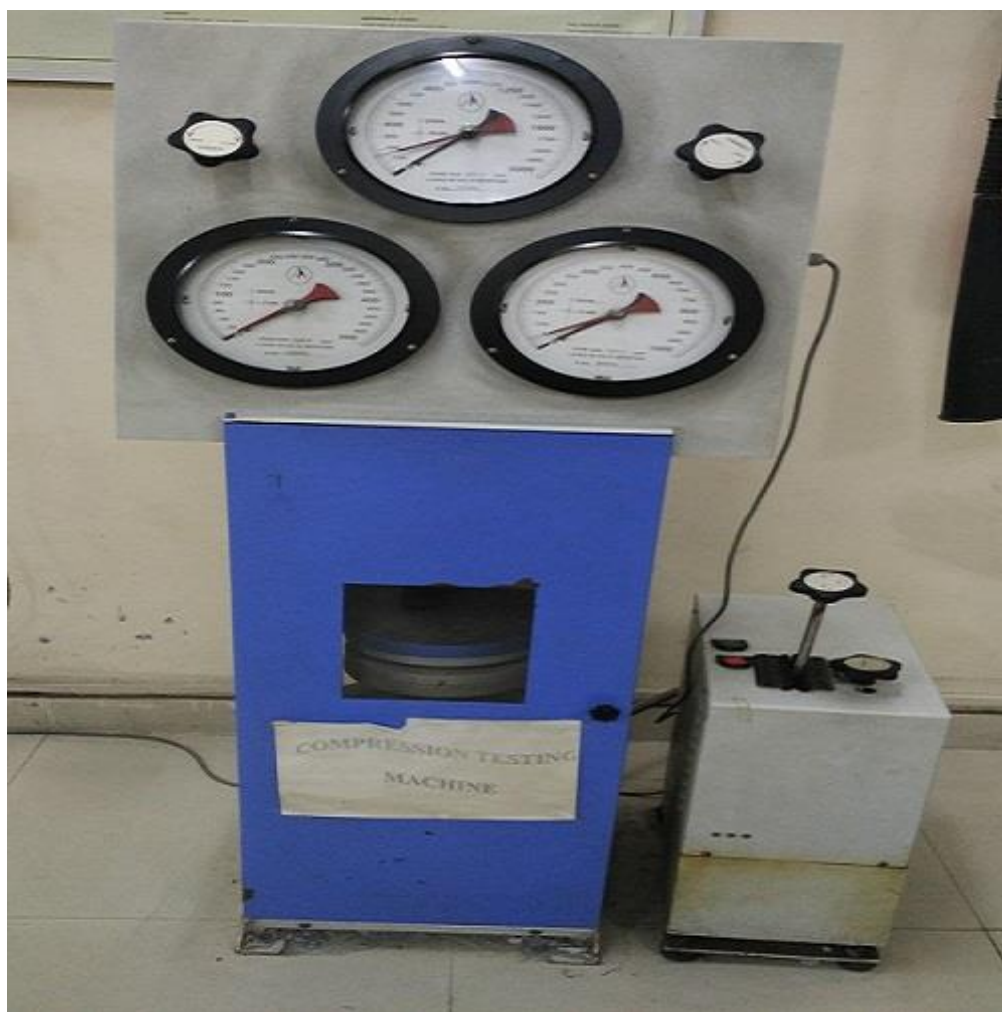
Figure shows compression testing machine used for test
