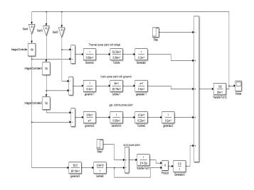
Fig-2:block diagram of single area multi source LFC system
